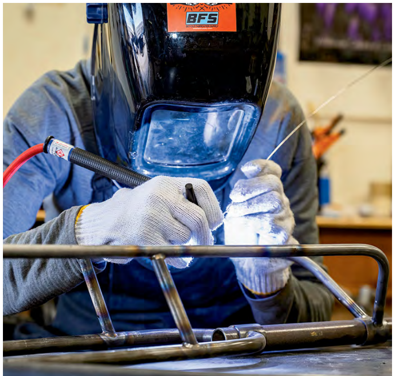
• [Below] Besnia TIG welds a steel truss fork designed to carry bolt-on, integrated panniers. Nearly all Goodday bikes have expansive cargo-carrying capabilities.
