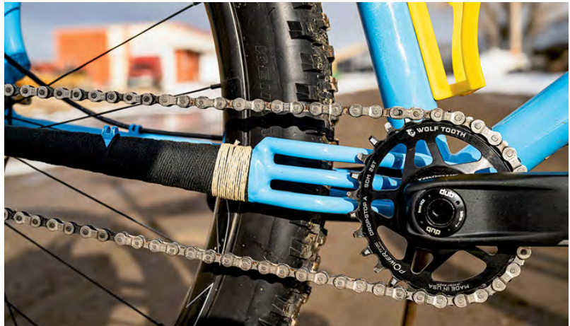
• [Above] The idea for this triple yoke chainstay, Besnia says, came to him in a dream and is an elegant solution for keeping cable routing clean.
